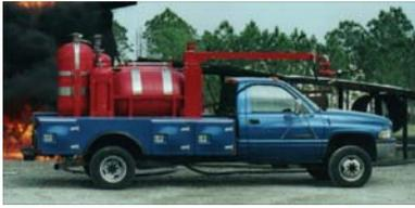
*U.S. Air Force Research Laboratory prototype of a portable, skid-mounted fire fighting system*
