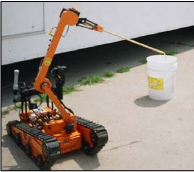
A robot by Allen-Vanguard Corp. is used to dip a pH test strip into a staged container of chemicals.
